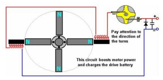
Here, two electromagnets are driven by the battery via Robert's 4-arm commutator which is mounted on the rotor shaft. Some of the recommendations given by Robert are the opposite of what you would expect. For example, he says that a single rotor construction tends to be more electrically efficient that one where several rotors are mounted on a single shaft. Robert is against the use of reed switches and he recommends making one of his commutators.
